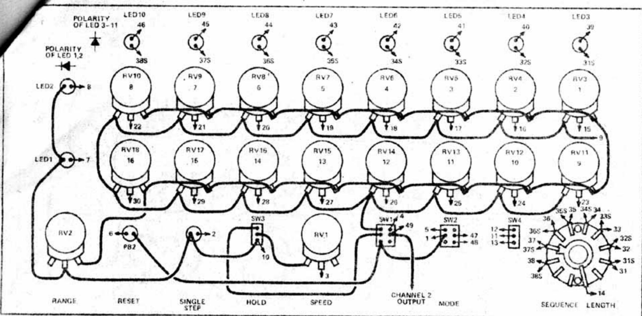
Fig. 5. Wiring of the front panel.
